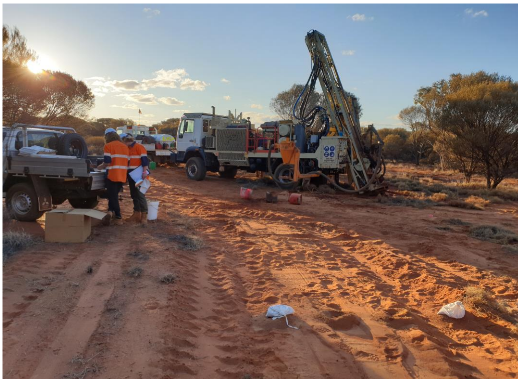
Photo 1 – Air-core drilling at the Valdez Prospect of the Leinster Nickel Project
