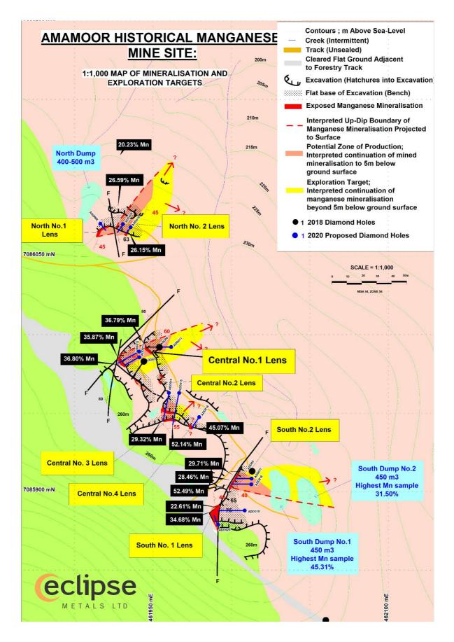
Figure 1: Amamoor Geological Map showing Proposed Diamond Drill Hole locations
