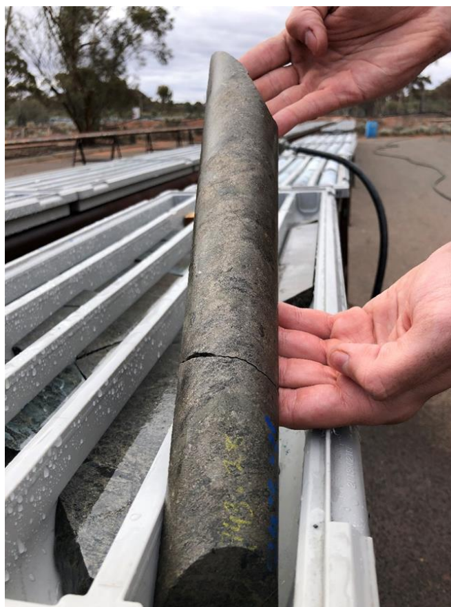
Figure 1: MDD339W4 core photo showing a section of massive nickel sulphides
