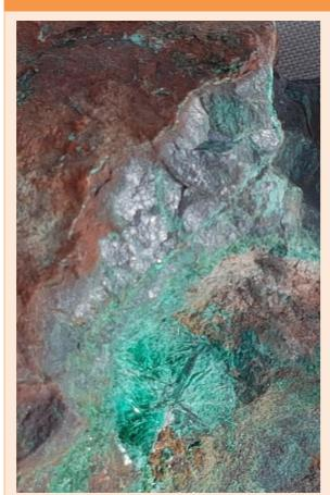
Note: Sample 11508-20200814\_100309 which is malachite and chalcocite believed to represent massive sulphide mineralisation (vein) occurring as supergene-oxide zone mineralisation in the stockpile.
