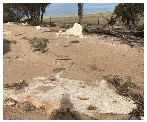
Figure 6 - Exposed in-situ kaolinized granite from location NB9
