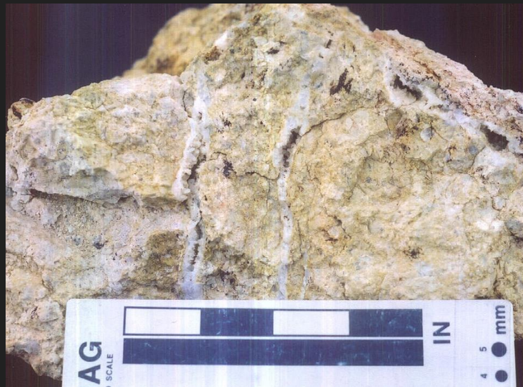
Hand specimen from Arrowhead Mine Site Steam heated advanced argillic alteration & vuggy quartz
