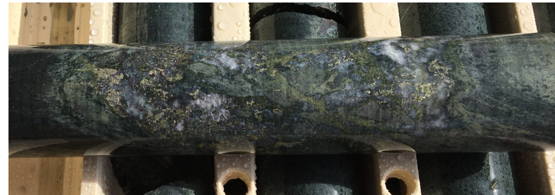
Figure 1. The best intersection of visual chalcopyrite observed in core from the mineralised zone (423m to 438m)
