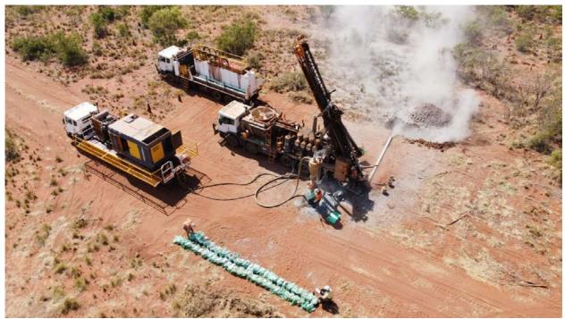
Figure 1 - Recently completed RC drilling at Cummins Range
