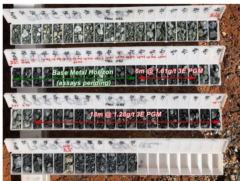
Figure 4 - Drill chip tray for hole PRRC083
