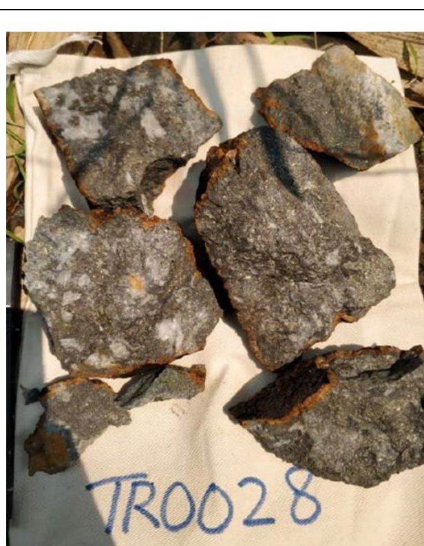
Figure 3 Sulphide rich fine grained volcanic which assayed 5.1g/t Au, 26g/t Ag, 204ppm Mo, 551ppm As, 5% S.
