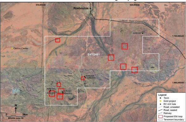
Figure 3: Andover layered mafic-ultramafic intrusive complex with Creasy Group drill hole collars and target locations for Azure's current electromagnetic program
