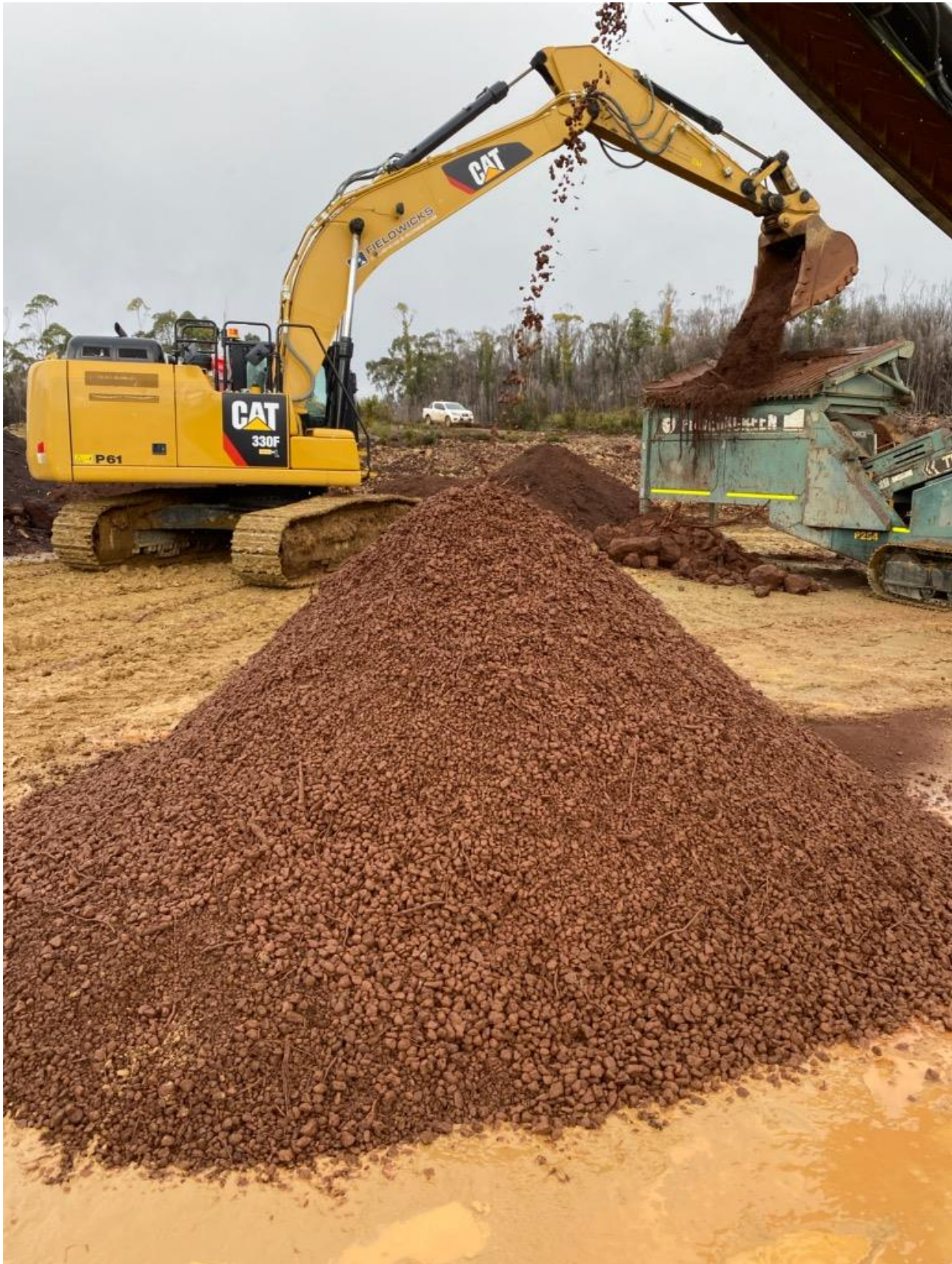
Figure Two | Dry Screening Iron Ore at the Riley Mine Site.
