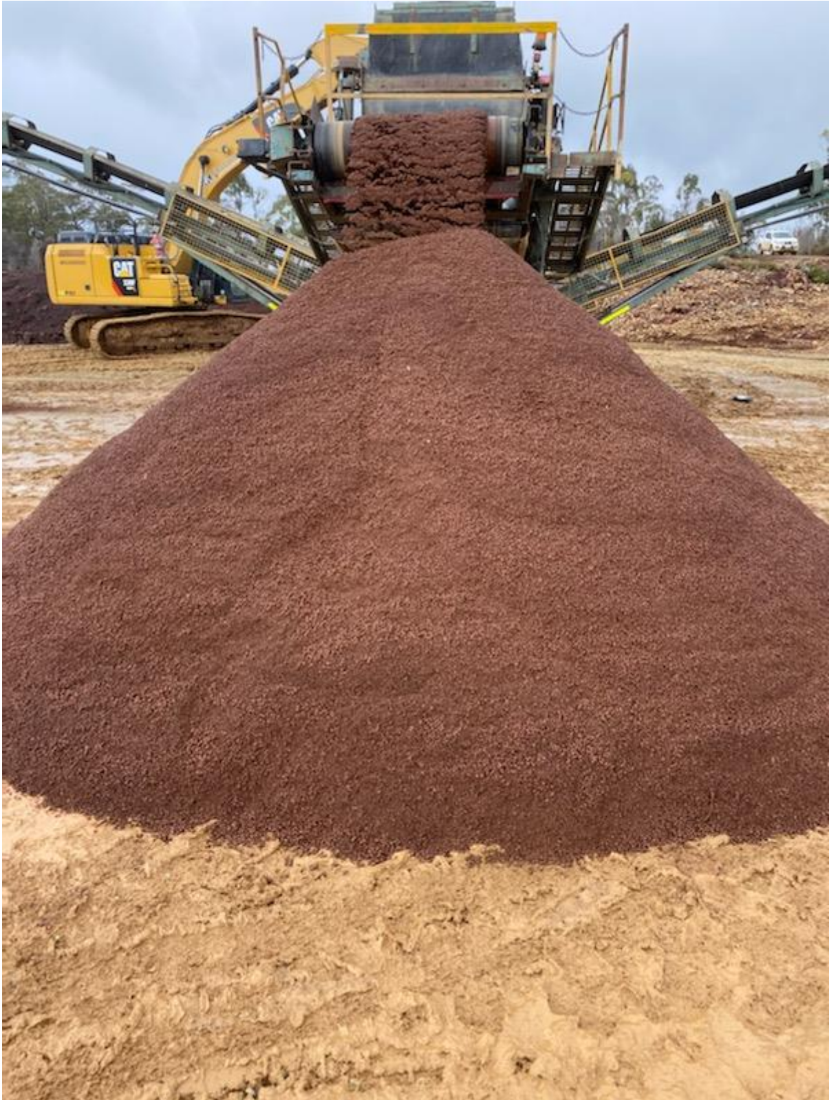
Figure Three | Another view of Dry Screening Iron Ore at the Riley Mine Site.
