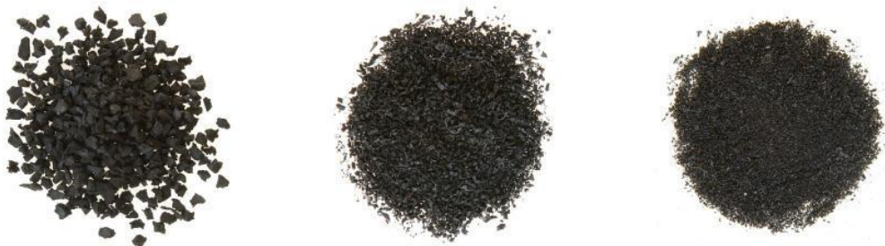
Image 1: Rubber crumb comes in various sizes depending on commercial applications. Finer sizes (far right) is 30 mesh and typically used in asphalt. Far left image is 2mm sizing for sporting and rubber moulds, with the image in the middle 10 mesh.
