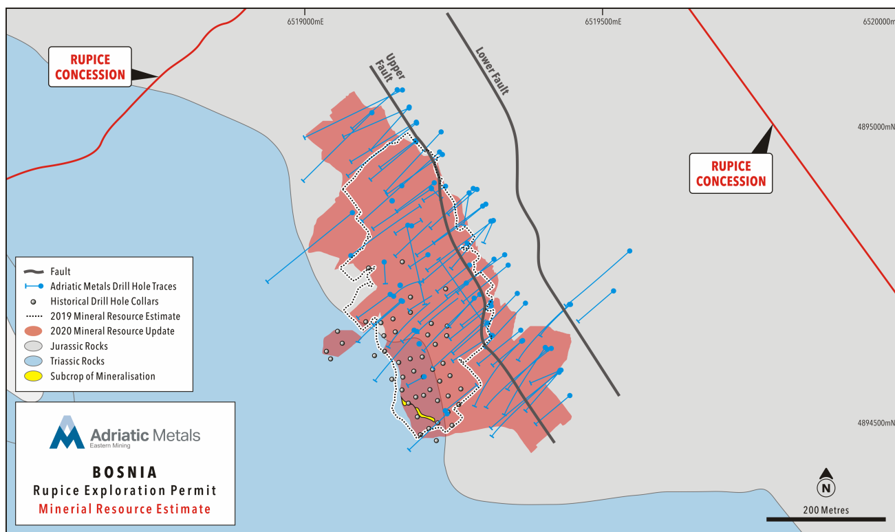
Figure 1 – Plan View of the New Ore Block Model Outline of Rupice vs 2019 Ore Block Model
