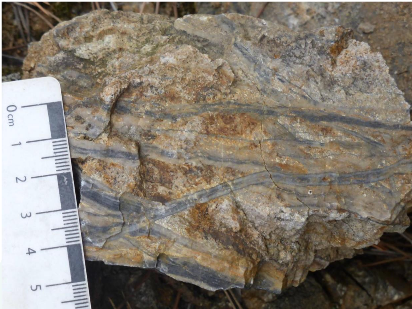
Figure 1 - sheeted and stockwork veining on the Sbor target
