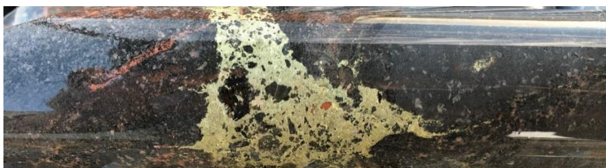
Figure 1. Chalcopyrite ( \text{CuFeS}_2 ) mineralisation within a quartz magnetite altered porphyry - HMSHDD001, 136.5m.
