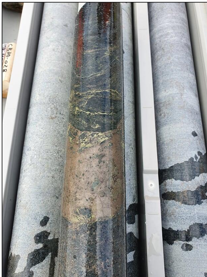
Figure 2. Semimassive and matrix style Ni sulphides (bronze colour) with stringer Cu sulphides (golden colour) in drill core (165m-165.5m shown).
