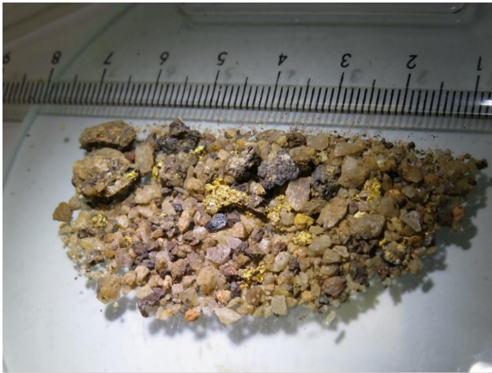
Visible gold within ferruginised quartz breccia (drill chips; OGGRC266; 9-10m; original assay 830.4g/t Au with a repeat of 757.9g/t Au)
