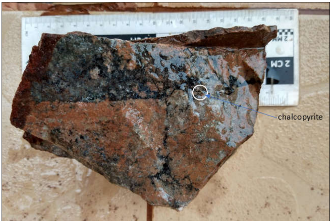
Figure 2: Sakaar Project - sample showing visible sulphide, K-feldspar and tourmaline alteration in a volcanic breccia
