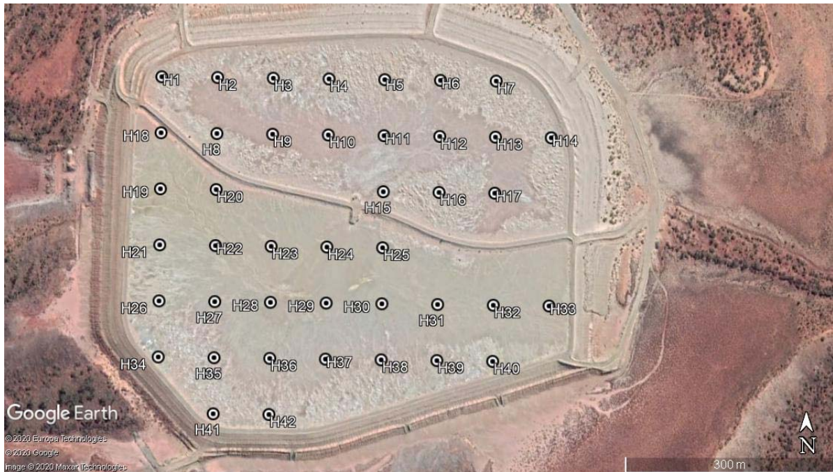
Figure 2 – Proposed drill hole location and pattern for HanTails TSF
