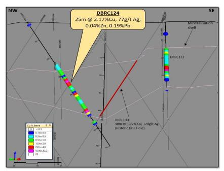
Cross section, looking towards the northeast, through hole DRBC124 showing assay results coloured by Cu % (see legend inset). Historically drilled holes are indicated by faint grey trace. The interpreted position of mineralisation is indicated by the pink outline.
