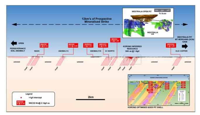
Long section of BIF exploration prospects located north and south of the Korong Resource. Inset is a 3D image of Dacian Gold's Westralia mining operation to scale with the long section sourced from DCX's ASX announcement on 13 September 2018
