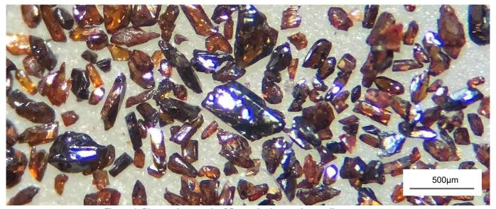
Figure 1. Photo-micrograph of Sovereign's premium rutile concentrate.
