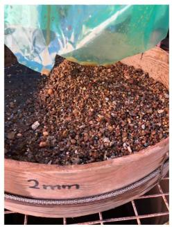
Figure 5 & 6. Left: Trommel screen processing the raw material & Right: +2mm oversize material
