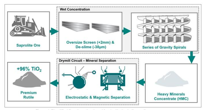
Figure 4. Simplified flowsheet developed for the Kasiya bulk metallurgy program.
