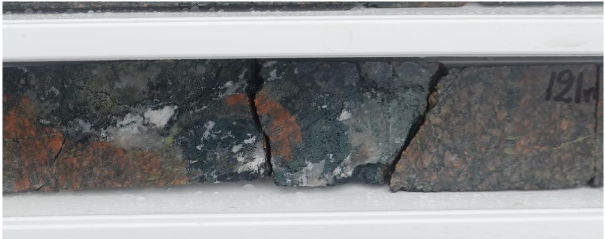
Figure 4: Close up of drill core from hole KKODD011 – 120-121m (7.18g/t Au) - altered feldspathic intrusive and mafic volcanic.
