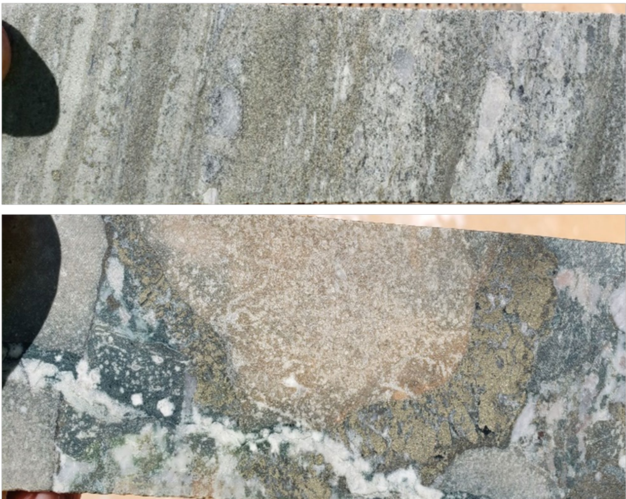
Figure 4: Core photos showing zones of strong sulphide mineralisation marked by strong multi-element geochemistry with sporadic high grade gold intersections in EL20DD332. Top - banded pyrite (198m downhole). Bottom - pyrite alteration rim around Felsic Volcanic rock fragment in Intermediate breccia with quartz carb veining (247m downhole).
