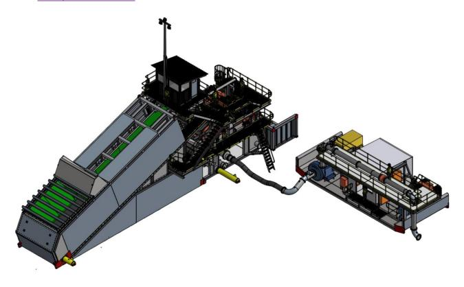
Figure 1 Conceptual image of Coburn's proposed in-pit dozer mining unit configuration
