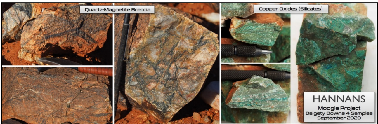
Figure 4. Photographs of outcropping quartz-magnetite breccia and oxide copper (silicates) from the Dalgety Downs 4 Prospect, Moogie Project.
