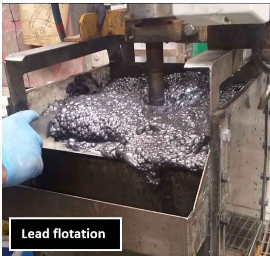
Figure 7. Lead -silver concentrate produced from bulk lead flotation test
