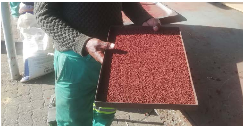
Figure 2: Successful agglomeration of by-product iron ore fines at Drytech
