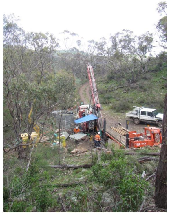
Figure 2: Diamond Drilling at Dead Horse Reef, QRD005
