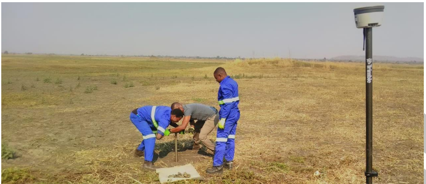
Figure 4. Sovereign's field team hand-auger drilling for rutile.
