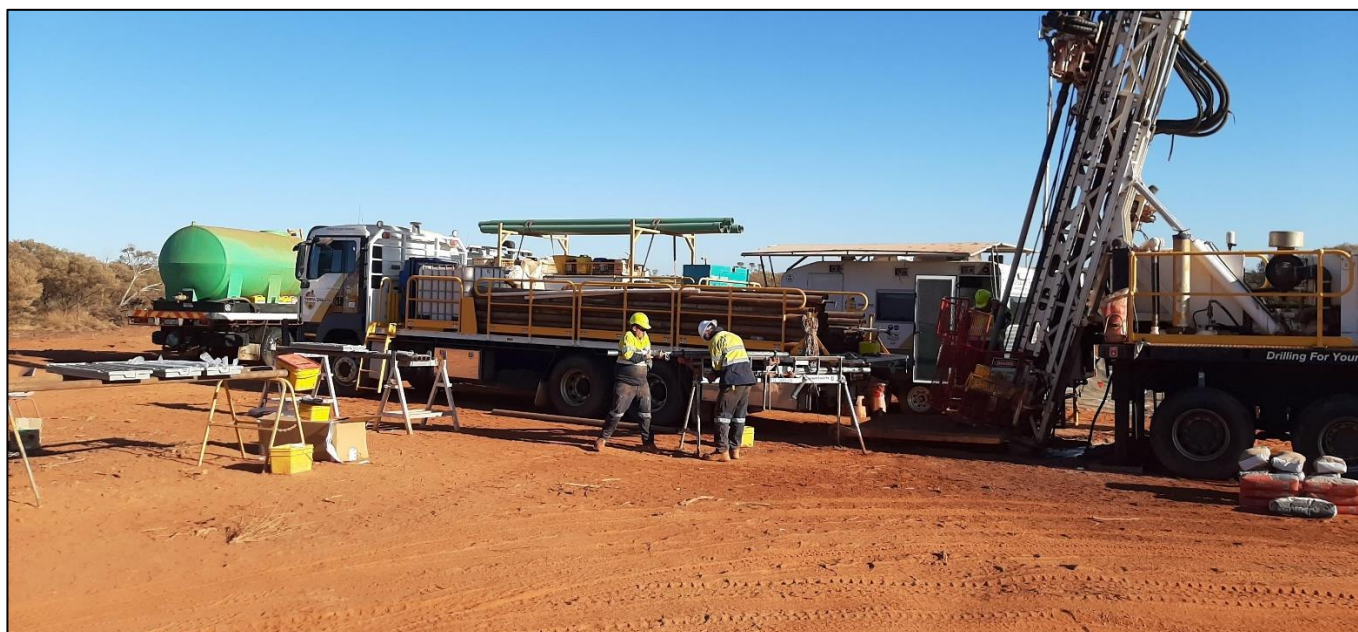
Figure 1 – Diamond drilling at the Flushing Meadows gold deposit in July 2020 to acquire data and samples for comprehensive geotechnical, hydrogeological and metallurgical test work.
