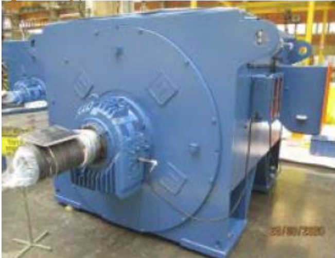
Figure Twenty | SAG Mill motor
