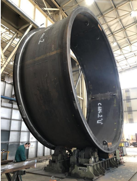
Figure Eighteen | SAG Mill shell
