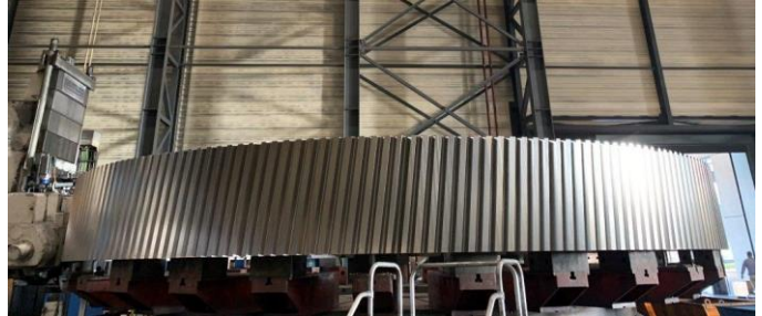
Figure Nineteen | Ring gear and mill head
