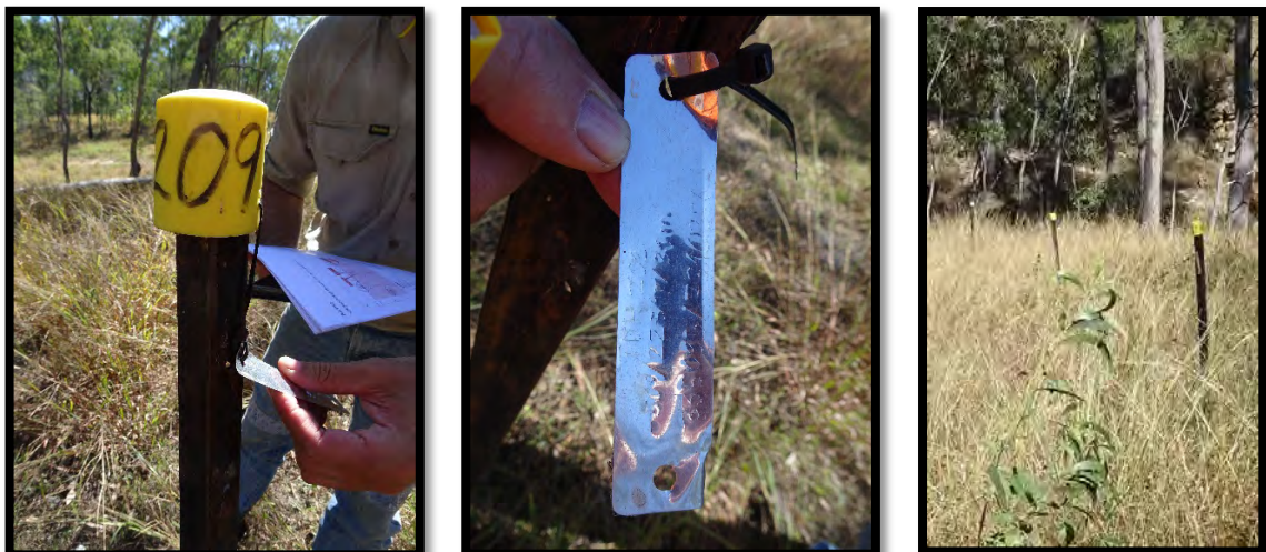
Figure 11-1: Example of RC diamond hole markers comprising plastic-capped steel pegs with aluminium tags. The right-hand figure shows how the yellow caps make drill lines easily identifiable, even in tall grass.
