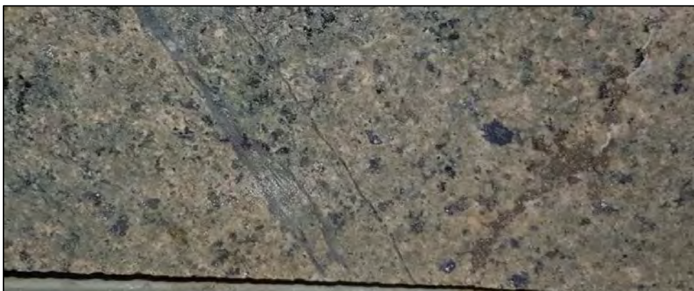
Figure 6-9: TDH115 (19.5 m) showing intense feldspar-sericite alteration and pyrite-molybdenite (black spots) vuggy infill. Field of view ~10 cm. (Source: XXXX Gold, Damien Keys).
