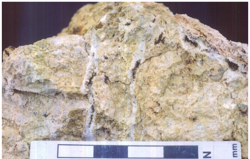
Figure 5: Hand specimen from Arrowhead Mine site: steam-heated advanced argillic alteration & vuggy quartz
