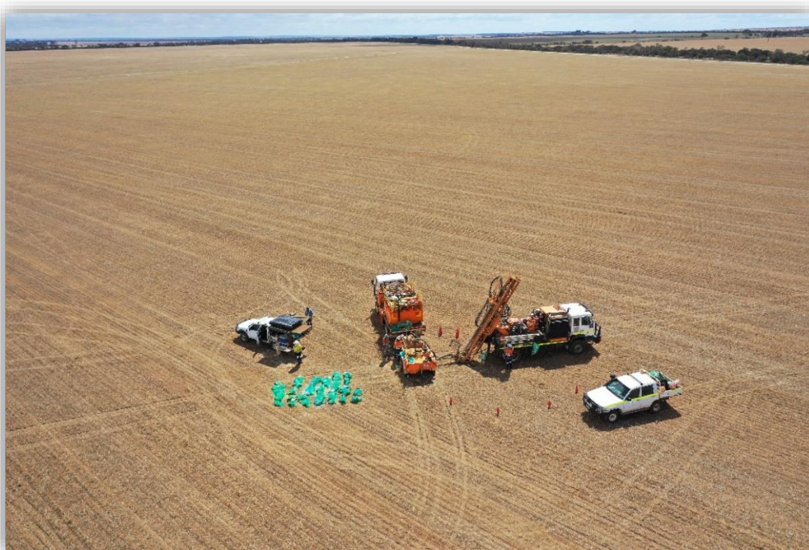
Figure 7: Air core drilling at Crossroads prospect March 2020 with 'Low Impact Rig', Burracoppin Gold Project
