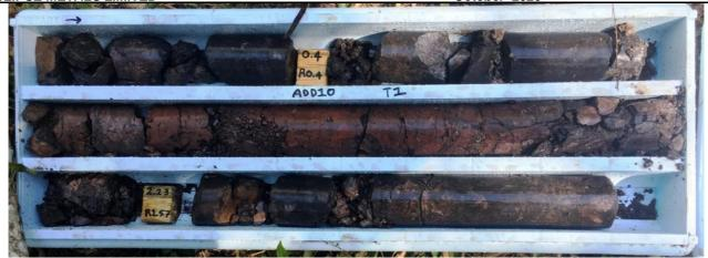
Photo 1: Northern Workings drill hole ADD010 - 0 to 2.74m, strongly fractured manganese mineralization with minor silicified japer fragments.
