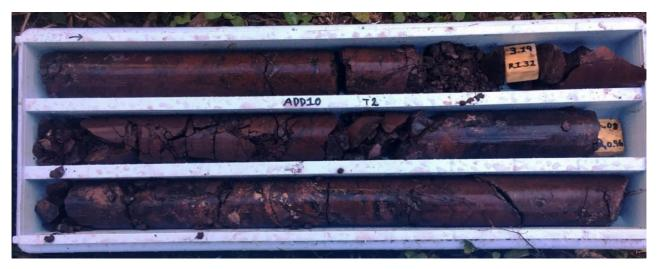
Photo 2: Northern Workings drill hole ADD010 – 2.74m to 5.1m strongly fractured manganese mineralization with minor silicified japer fragments.
