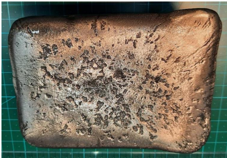
Figure 1: 99.53% Dy Metal Produced at the Ziron Tech Pilot Plant
