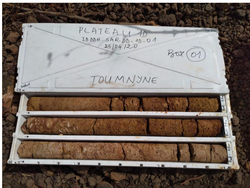
Figure 5 – Example diamond drill core from a hole from the 2020 Sarmin drilling program
