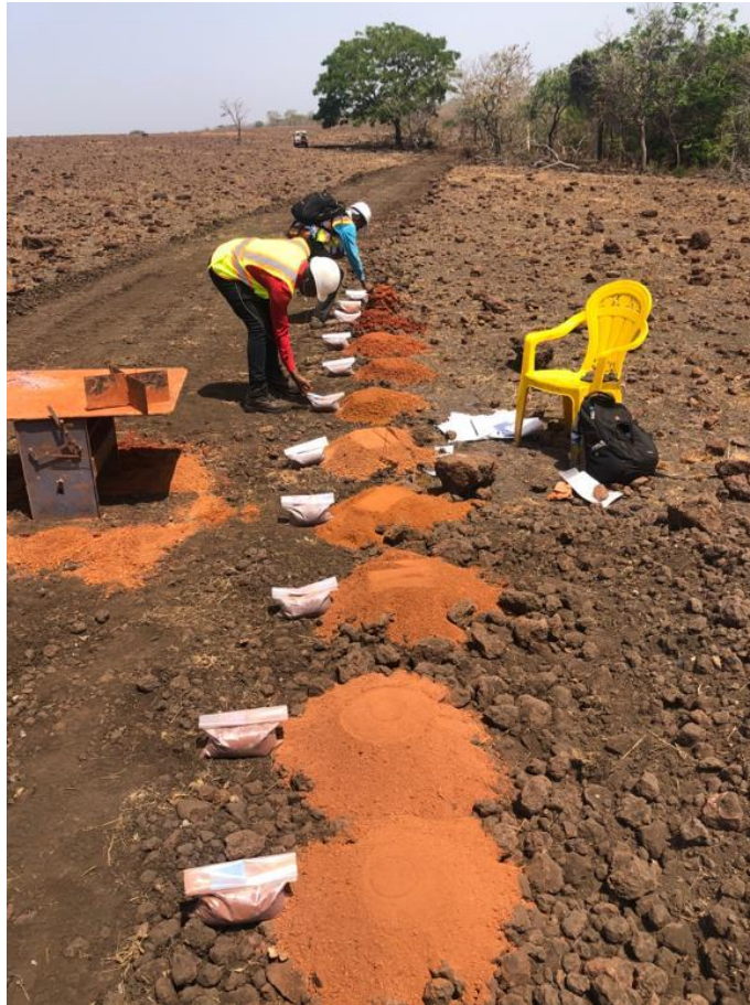
Figure 4 – Meter interval drill samples are logged, weighed, split and sampled for analysis. Sample rejects with the accompanying sample aliquots shown in the photo
