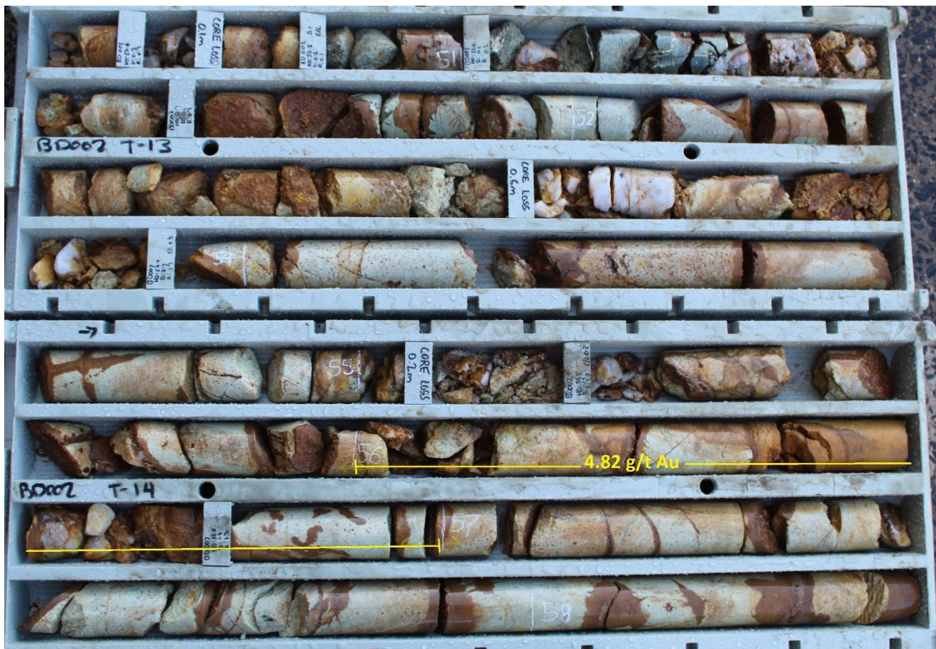
Figure 4: BD002 Core Tray which includes the 1m interval @ 4.82g/t gold from 56m
