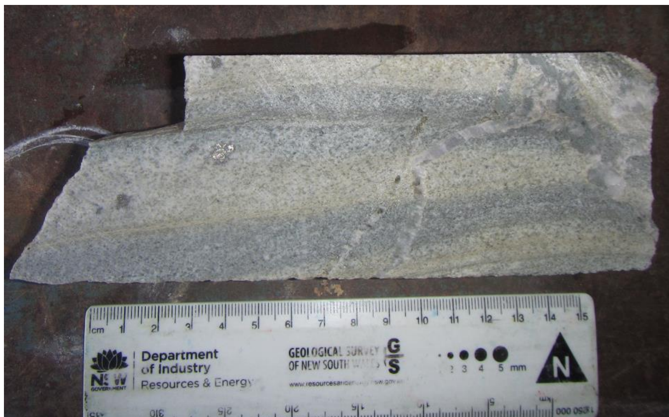
Figure 3: BD001 at 152.8m displaying strong sericite altered sandstone with pyrite clots
