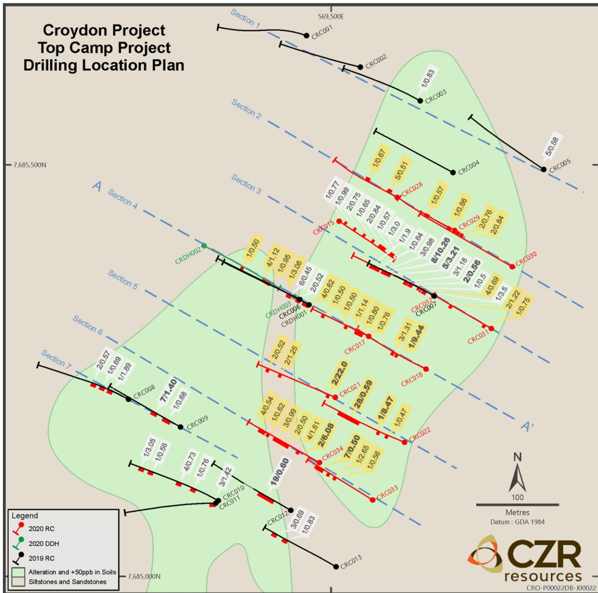
Fig 1. Location and down-hole traces of the diamond and RC drill-holes at Top Camp from 2019 and 2020 with significant intercepts (cut-off >0.3g/t and including 1m>0.5g/t Au) in each drill-hole reported as metres at grams/tonne Au. Previously reported results are in a white background (CZR releases to ASX; 6 February 2020 and 2 September 2020) and new results in a yellow background. The map also shows the traces of section lines 3 and 5 that are presented in cross-section on Figs 2 and 3 below.
