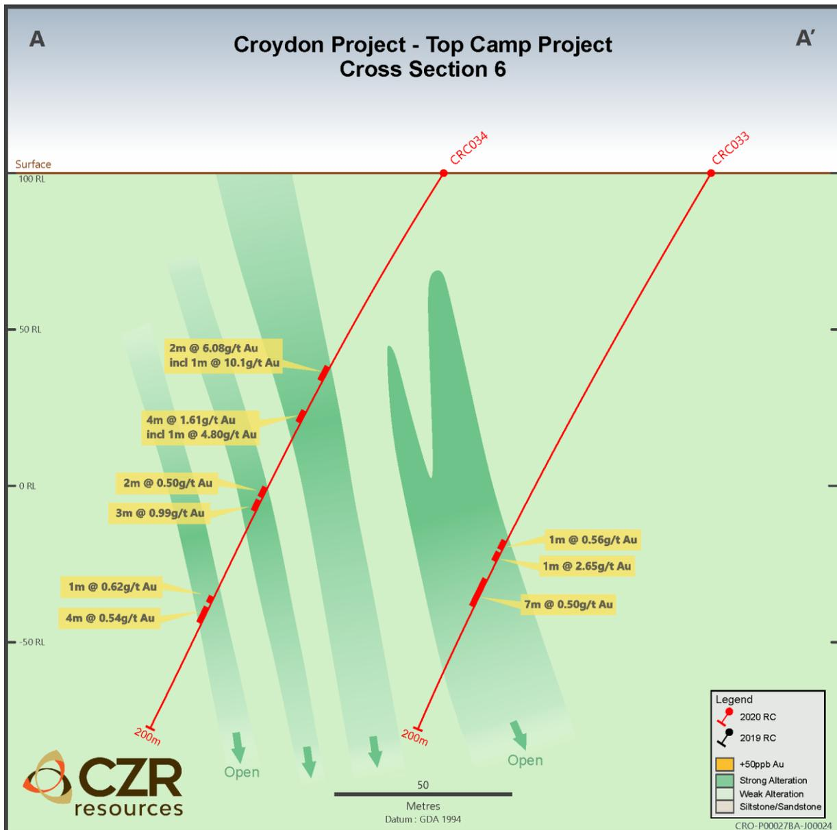
Fig 3 Section 6 from Fig 1 showing the significant down-hole intercepts (cut-off >0.3g/t and including 1m>0.5g/t Au) in each drill-hole reported as metres at grams/tonne Au.
