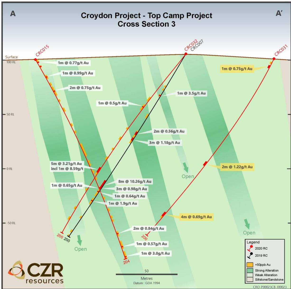
Fig 2. Section 3 from Fig 1 showing down-hole traces marked with significant downhole intercepts (cut-off >0.3g/t and including 1m>0.5g/t Au). Previously reported results are in a white background (CZR releases to ASX; 6 February 2020 and 2 September 2020) and new results in a yellow background.
