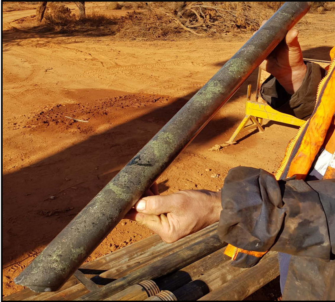
Massive Ni-Cu Sulphide from RKDD027 from 168.5m, NQ2
