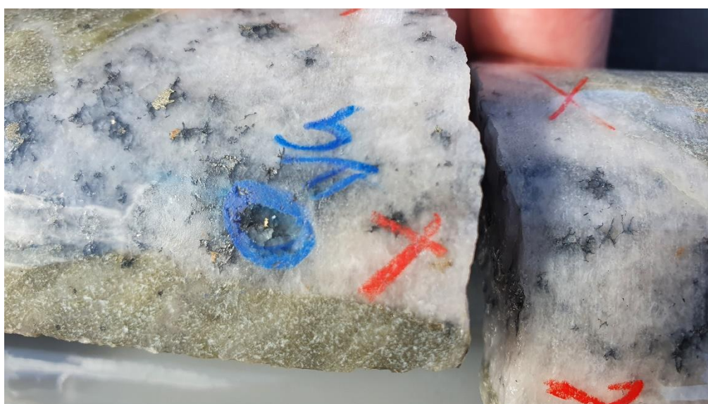
Figure 1. RXDD004 – 202.2m: Strong sericite-altered granite and quartz-stibnite-gold vein.
