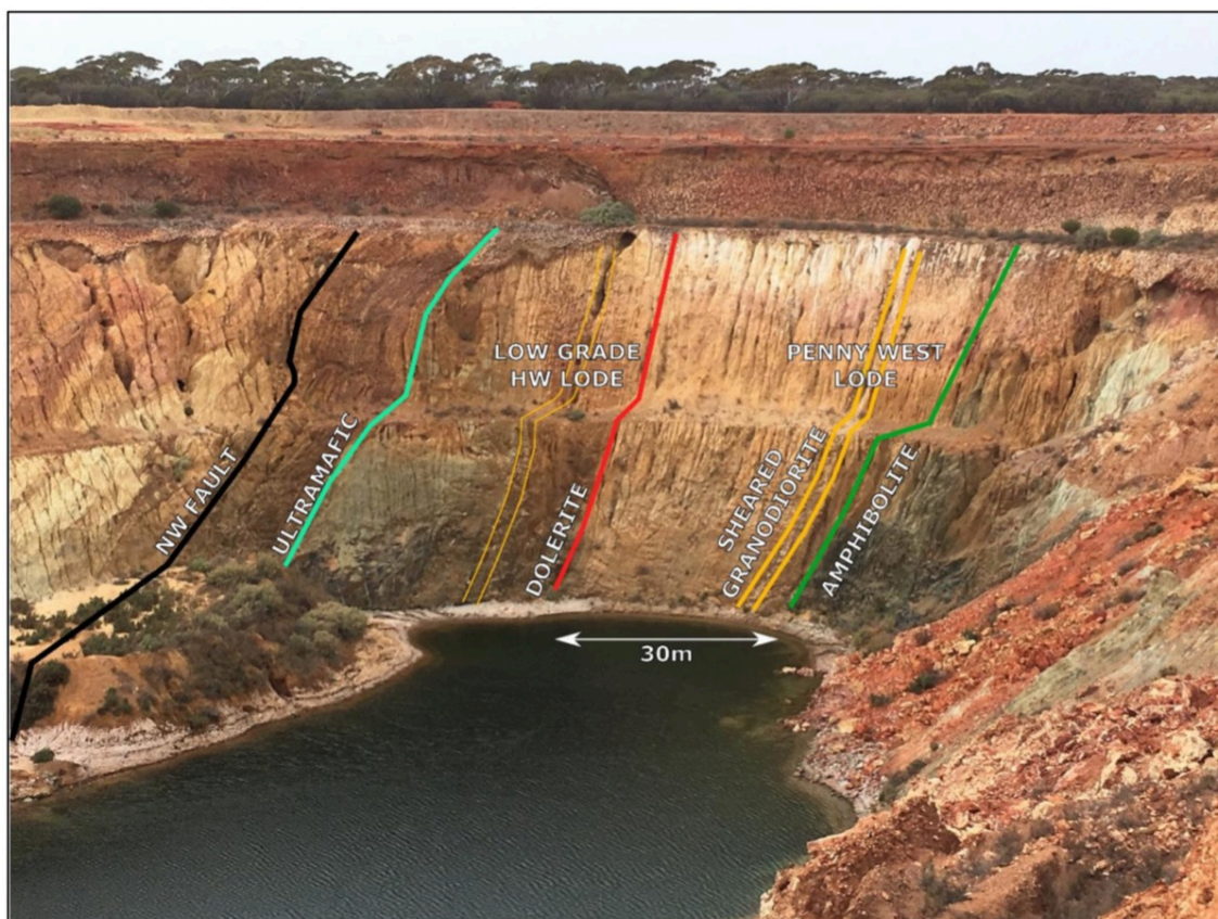
Figure 2: South end of Penny West Pit noting high-grade and low-grade lodes (from ASX:SPX, 29 August 2019)
