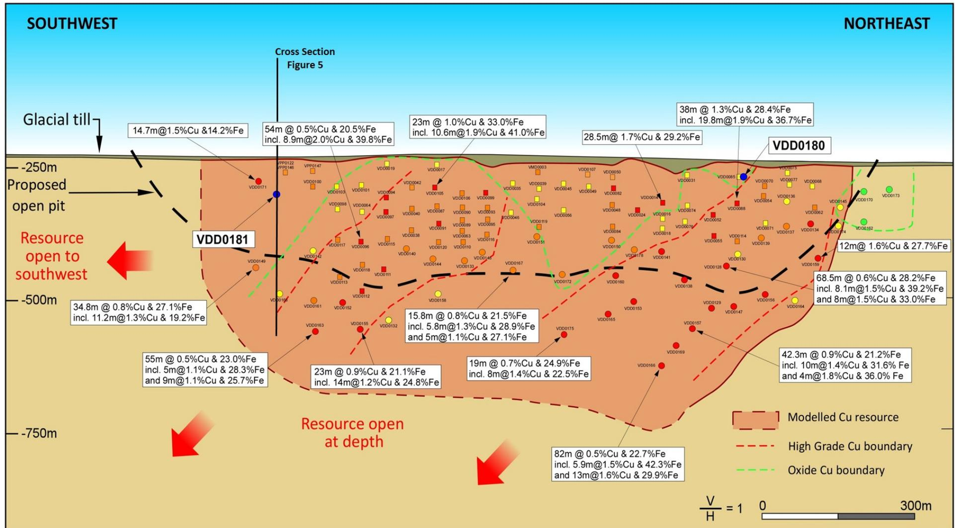
Figure 5: Cross-section showing the actual depth of VDD0181, compared to the planned target depth.
