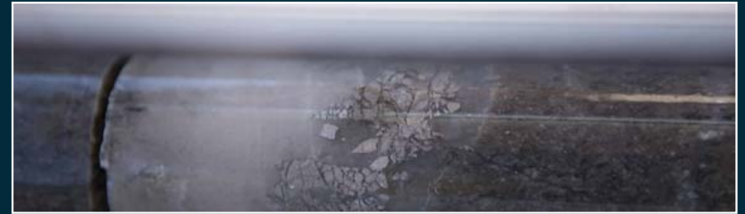
Gruyere drill core, 14GYDD0008 - Arsenopyrite vein in porphyry
