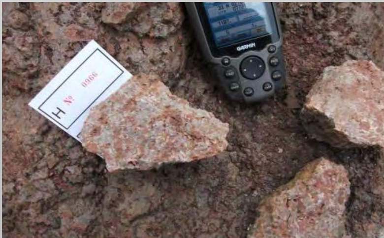
Bauxite sample 63.79% \text{Al}_2\text{O}_3
