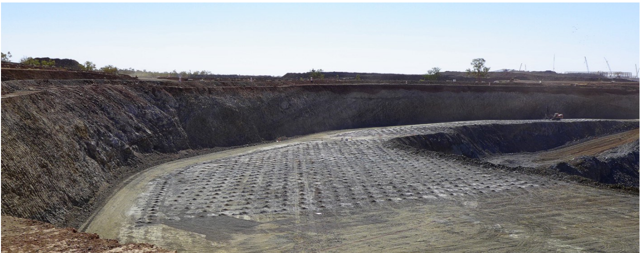
Figure 12: Top 2 images show LM1 and LM2 Pits being mined concurrently. Bottom image shows blast pattern completed and ready for loading.
