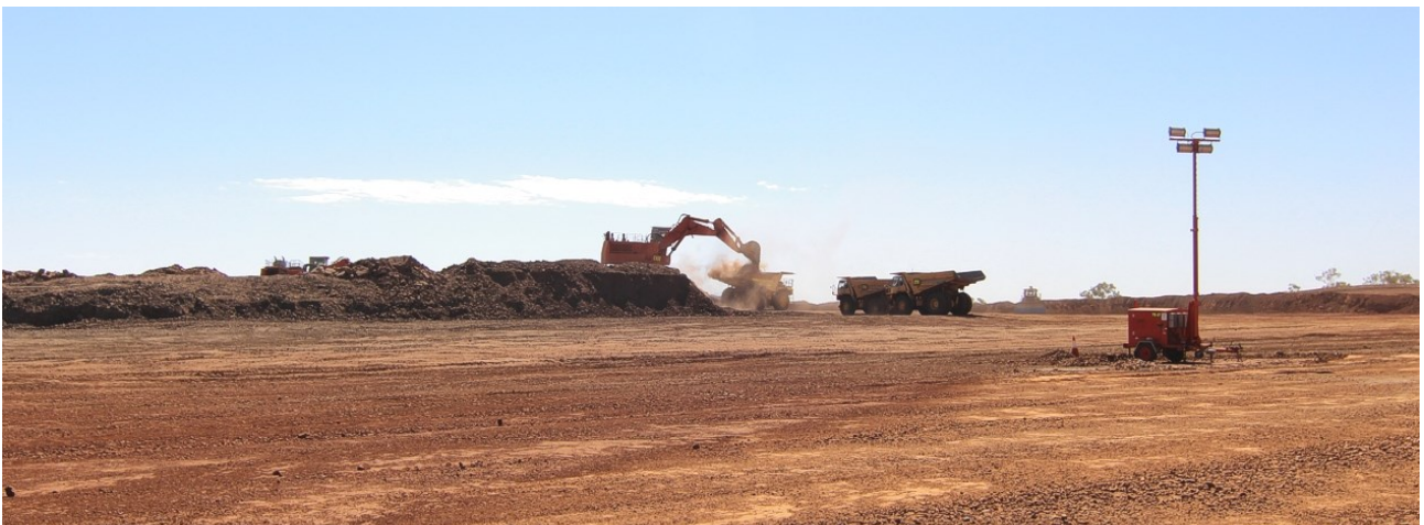
Figure 14: Above images shows triple benching (mining 3x 2.5m flitches at once) in waste areas to optimise mining costs. Below images shows Rocklands South Pit (RS1) commencing.
