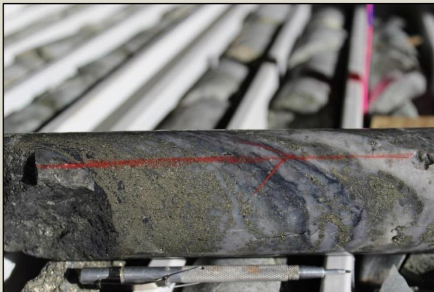
First drill hole into the Junction prospect also intercepted broad intervals of low-level copper mineralisation in phyllic over propylitic alteration:
