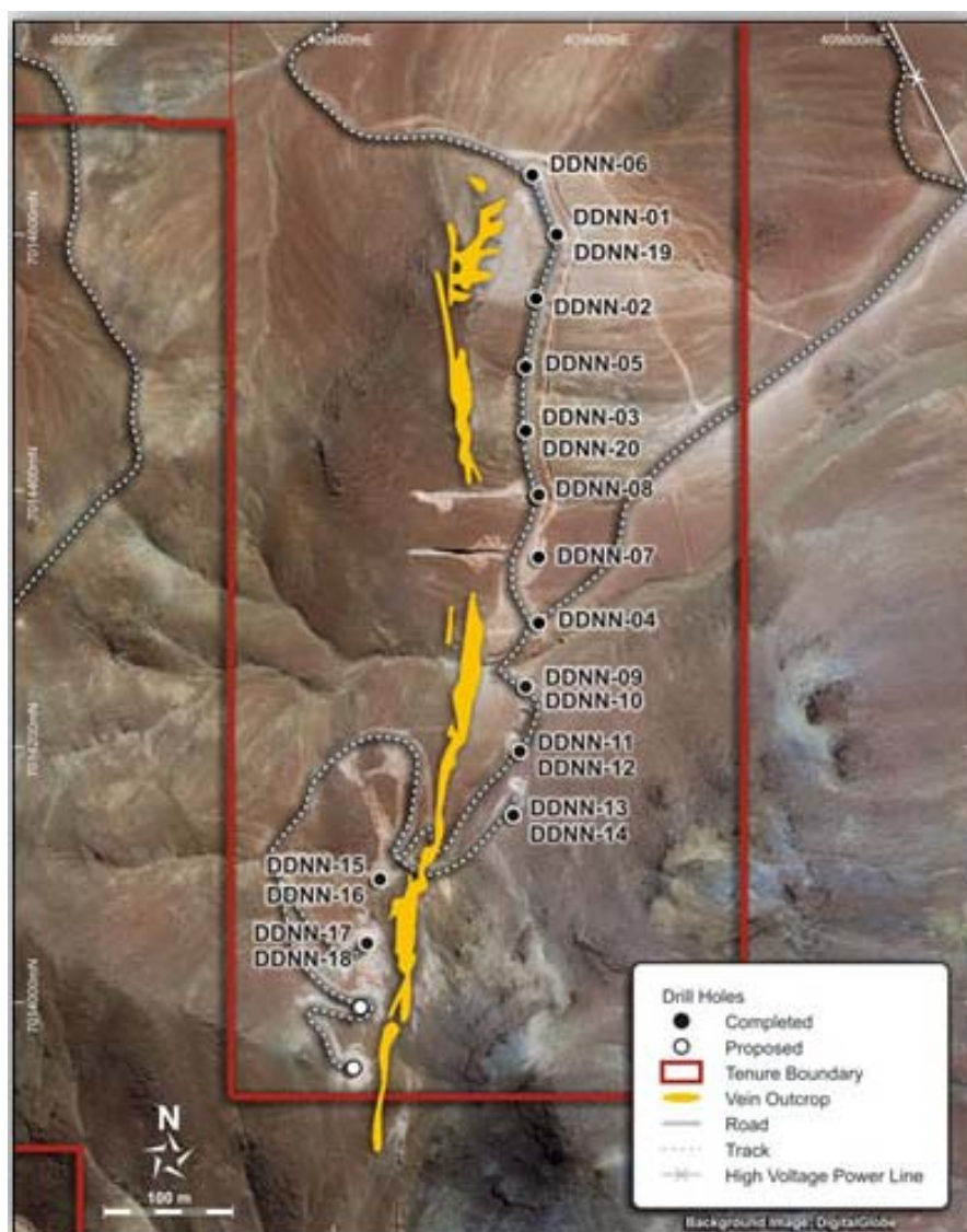
Figure 24: Location of diamond drill collars near the Nany vein system. The locations of the trenches are also visible.
