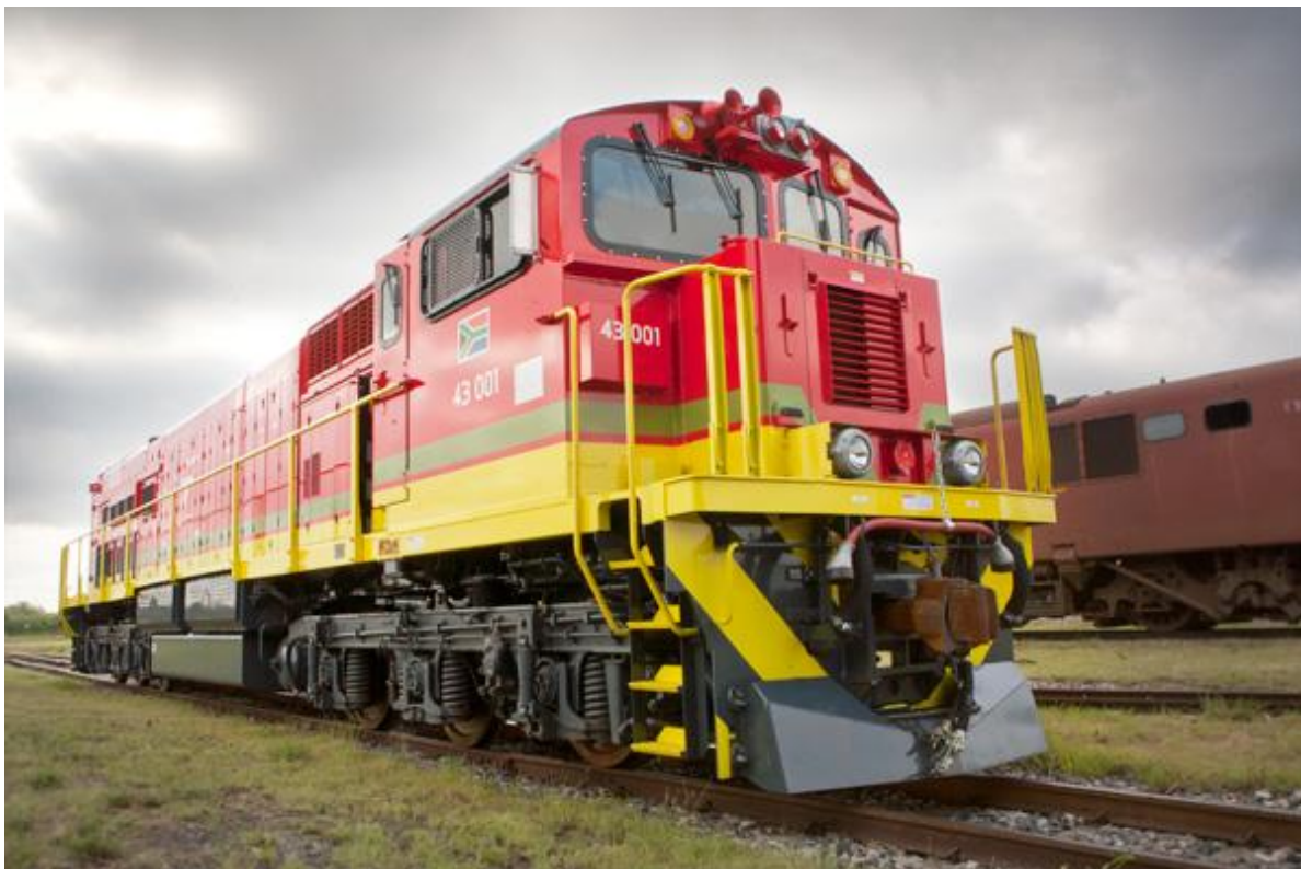
Figure 10: AC Traction Power Locomotive on six wheeled bogies
