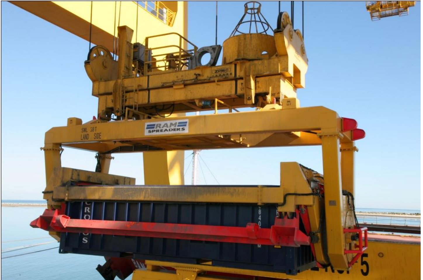
Figure 12: Half Height Container on rotating RAM spreader prior to discharging
